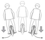
06. Turn by pressing harder on one pedal than the other, and by shifting your weight slightly.
