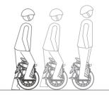
04. After you are able to comfortably glide for a few seconds, try gliding for 10-20 ft (3-5 m) with both feet on the pedals.
