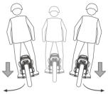
06. Turn by pressing harder on one pedal than the other, and by shifting your weight slightly.
