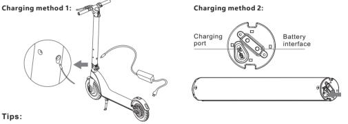
Remove the battery to open the silicone charging port, plug the charger DC plug into the battery charging port; plug the power cord into the charger, then connect the other port to the socket (100V-240V; 50/60Hz), and confirm the charger indicator is on normally
