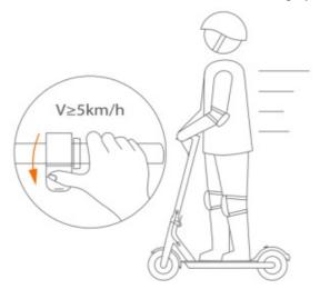
4. Release the accelerator and squeeze the brake lever for a sudden brake.
