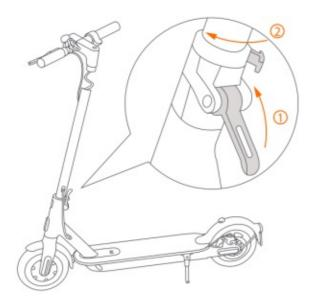
2. Install the handlebar onto the stem.
