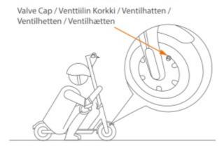
• Connect the extension nozzle to the tire valve stem.
