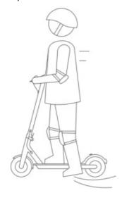
3. The accelerator initiates once the coasting speed exceeds 5 km/h.
