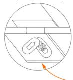
2. Plug the power adapter into the charging port.
